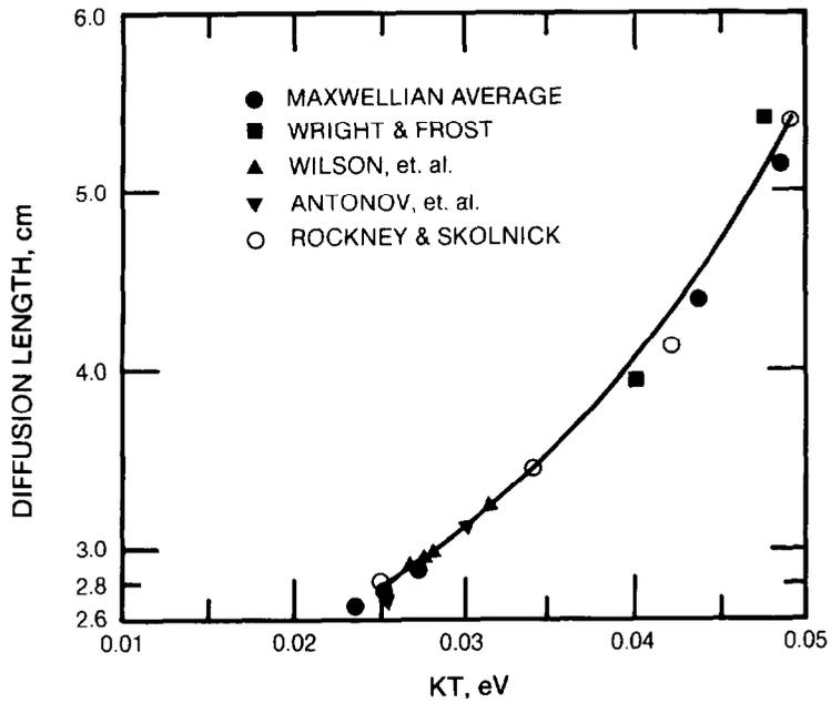
FIGURE 2. Comparison of measured and computed values of L, the thermal diffusion length of water, at elevated temperatures.
