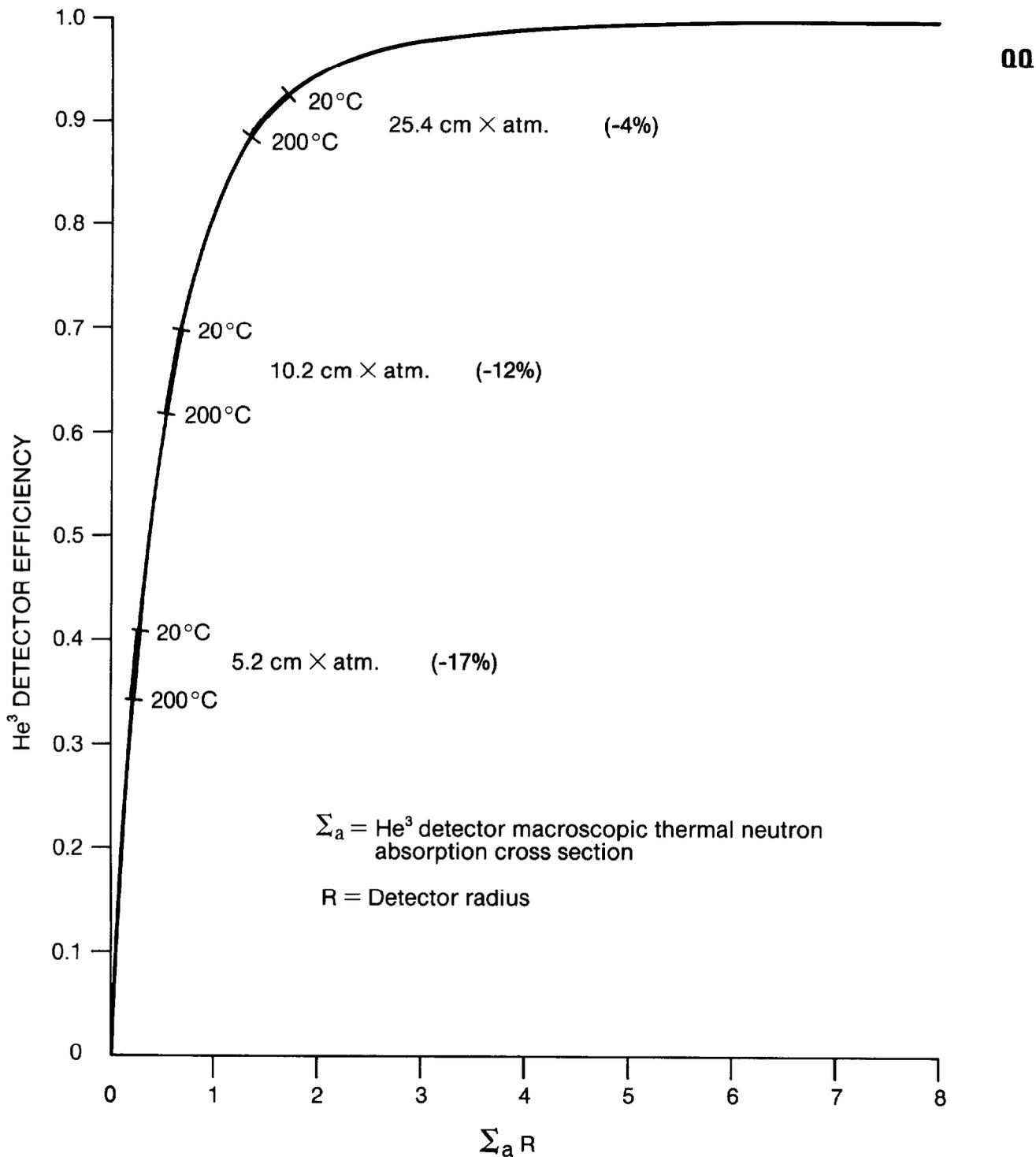
FIGURE 4. He<sup>3</sup> detector efficiency versus  $\Sigma_a R$ . See equation 11.7.27 from reference 11. One far detector is shown, together with two different near detectors.
