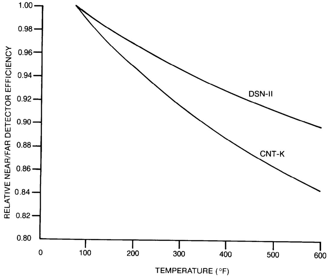
FIGURE 3. Relative near/far detector efficiency versus temperature for two different logging tools.
