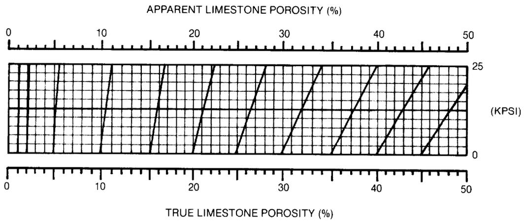
FIGURE 7. DSN-II formation pressure correction, at 75°F.
