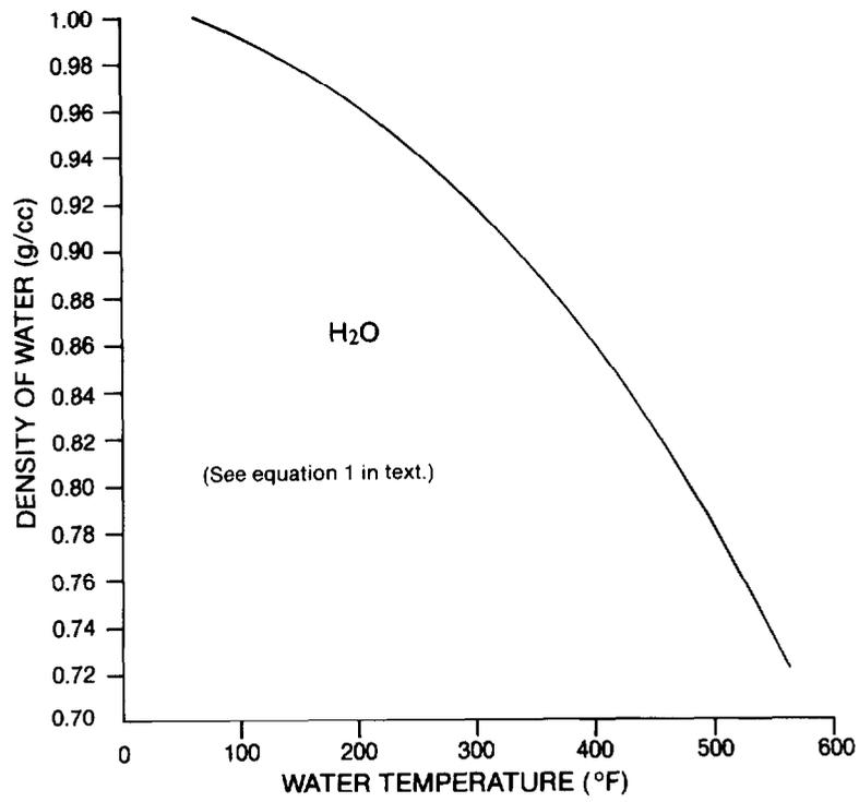
FIGURE 1. Density of water versus temperature.
