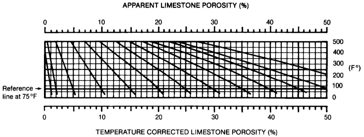
FIGURE 6. DSN-II formation temperature correction in waterfall format.
