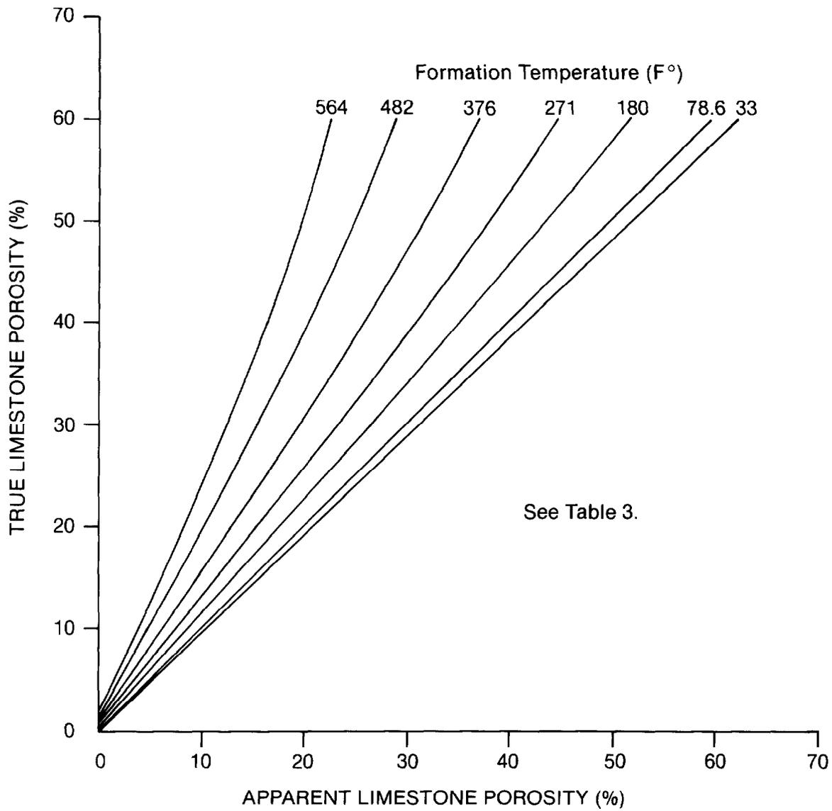
FIGURE 5. Apparent DSN-II porosity versus true porosity for temperatures from 33 to 564°F.
